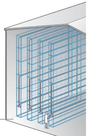
The highly sensitive, laser-based detector then measures the amount of smoke in the air. The measured smoke levels are compared to the 4 alarm thresholds set by the user. These alarm thresholds allow a staged response to any threat.
