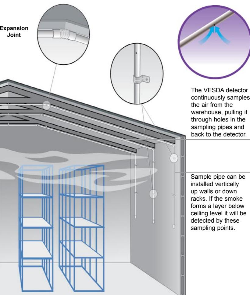
Sample pipe installed in racks will ensure the earliest possible warning of a fire that starts there.
